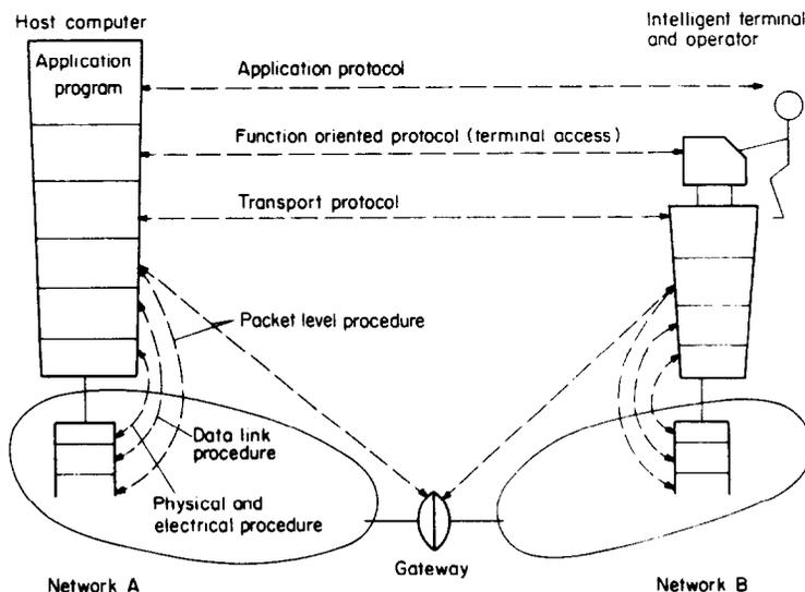
**Figure 2.** Overview of major functional levels for data communications between a host computer and a terminal through interconnected data networks.
