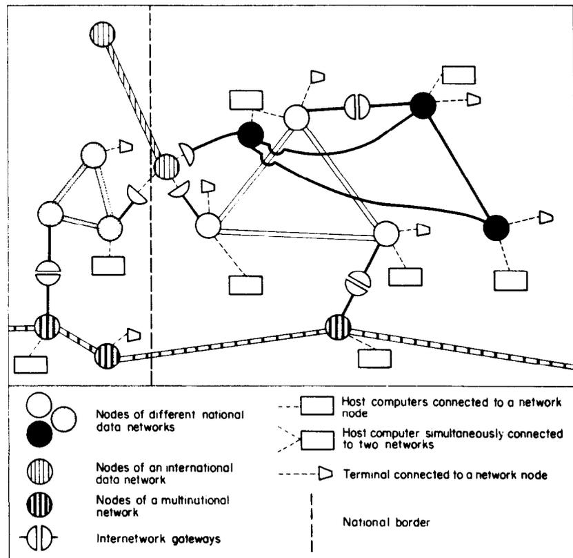
**Figure 1.** The possibilities for internetwork data communications.
